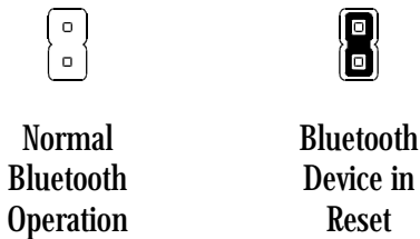
Figure 7 – JP12 Jumper Setting
