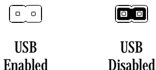
Figure 3 – JP13 Jumper Setting
